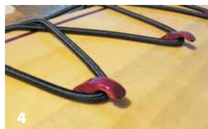
3 & 4—Purpleheart provides a nice contrast for the outline of the deck design and deck hardware. Everything is coated with 105/207 and finished with 5 coats of Z-Spar Captains Varnish.
