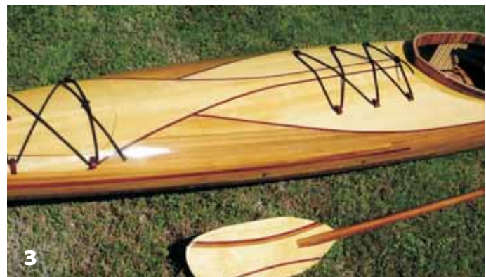
3 & 4—Purpleheart provides a nice contrast for the outline of the deck design and deck hardware. Everything is coated with 105/207 and finished with 5 coats of Z-Spar Captains Varnish.
